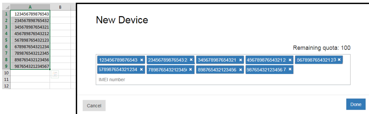
Figure 7: A list of IMEI numbers are copied from Excel and then pasted as new devices in the Mass deployment program list.
