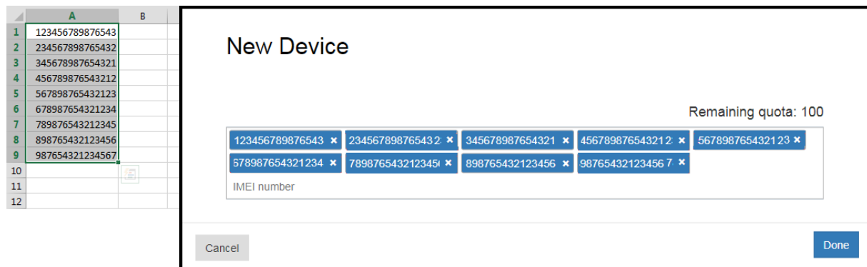
Figure 7: A list of IMEI numbers are copied from Excel and then pasted as new devices in the Mass deployment program list.
