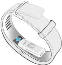
Insert the core into the wristband in such a way that the power key is inserted underneath the power key cover.
