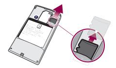
Remove the battery cover, then press the edge of the memory card and draw it outwards. Release and remove.
