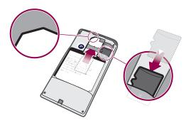
Remove the battery cover, then insert the SIM card and the memory card in the relevant slots.
