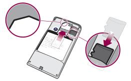
• Remove the battery cover, then insert the SIM card and the memory card in the relevant slots.
