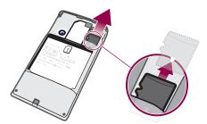
• Remove the battery cover, then press the edge of the memory card and draw it outwards. Release and remove.
