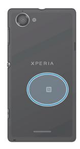
The location of the NFC detection area is not the same on all devices. When sharing data with another device using NFC, refer to the User guide of the other device for more information.
